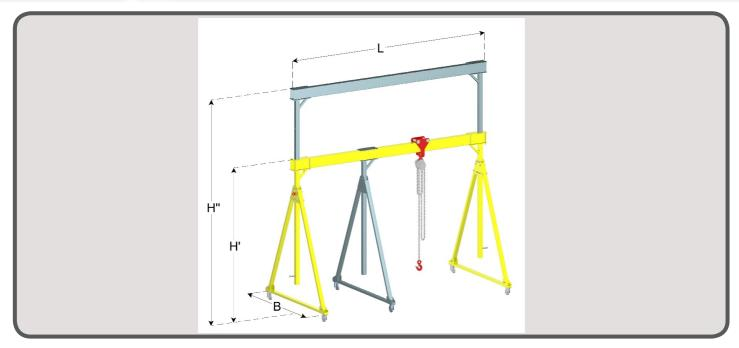
Light construction, Bolted joints, Easy assembly with 8 bolts between leg and beam, Assembly requires 1 to 3 people according to model, Flexibility of movement due to its light weight, Hollow-section gantry girder, Hoist trolley provided, Height under beam can be adjusted by single person, Dismountable in 3 elements, with foldable feet, Feet fold up for transport, White polyamide wheels with 2 locking wheels
